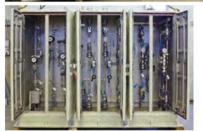
HIPPS system is a specific application of SIS (Safety Instrumented System) and is used in the Oil & Gas industry in order to provide protection for downstream equipment against overpressure or unsafe conditions coming from upstream.
